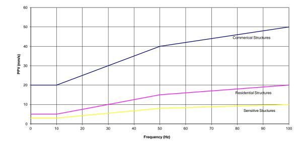
Figure 1 Baseline Curves Representing Short-Term Vibration Effects on Structures in Relation to Recorded Data
